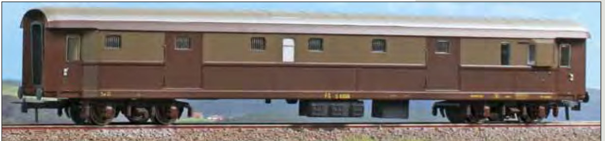
Bagagliaio FS Tipo 1946 (Dz 83000) in livrea castano e Isabella, carrelli FS AM. Type 1946 luggage car (Dz 83000) of the FS, two tone brown livery, Type FS AM bogies. Typ 1946 Gepäckwagen der FS (DUz 83000), castano-Isabella Lackierung, Typ FS AM Drehgestelle
