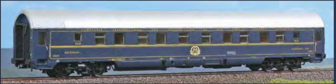
Carrozza letti UHansa 4581 con mantici e carenatura originale CIWL immatricolata presso il Parco DB. Sleeping car UHansa nr. 4581, owned by CIWL, with original ends and side skirt, registered in Germany. Typ UHansa Schlafwagen, Originallackierung bei der DB eingestellt.
