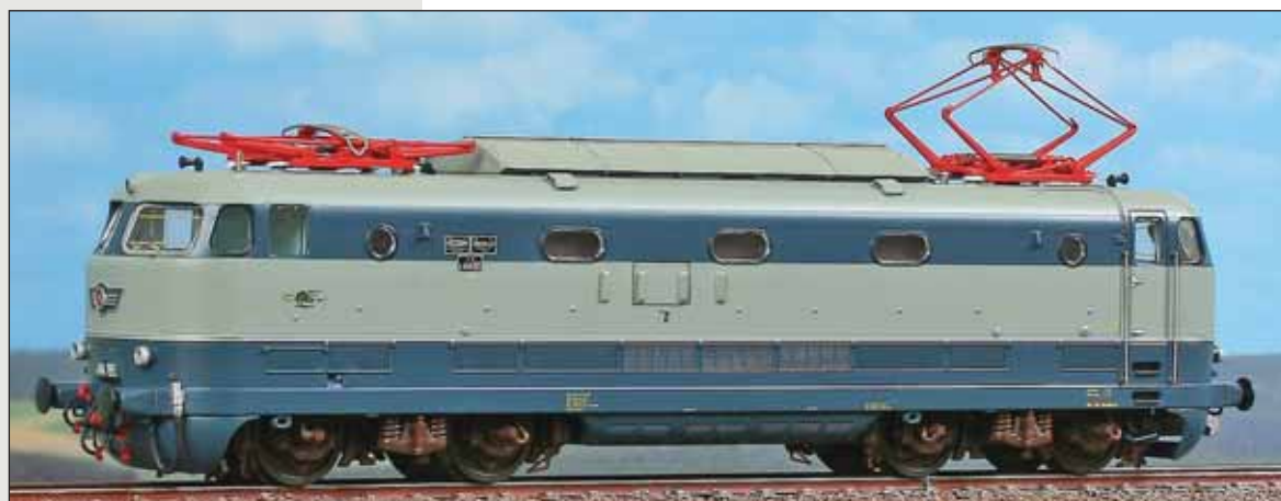
Locomotiva elettrica E.444.093 di II serie, senza baffo rosso, con modanature. Electric locomotive E.444.093, 2nd series, without red plank and with mouldings. Elektrolokomotive E.444.093, ohne rote Front und mit Zierleisten.
